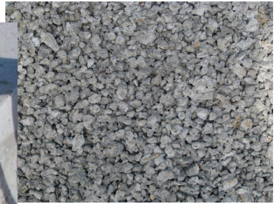
Pervious concrete is made without sand so water can pass through its pores
